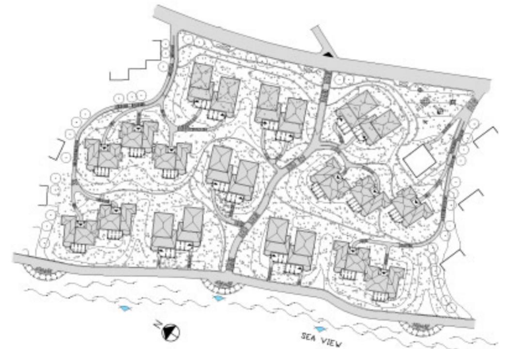
Site plan. The position of each house was determined on the site, in relation to the other houses, so as to ensure an open view of the sea.
